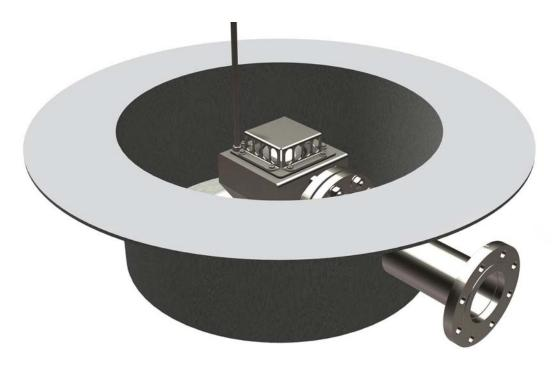
The SumpMaster<sup>TM</sup> is a sturdy sump valve designed to prevent product flow onto external floating roofs from drain system failures. The SumpMaster<sup>TM</sup> addresses several problems with traditional check valves, including more effective sealing at the potentially lower pressures encountered during a drain system failure, and not restricting drain flow rates calculated during the design of the floating roof.
